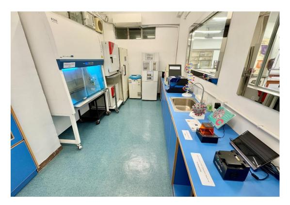
The biotechnology laboratory is equipped with advance biotechnology equipment including over 40 micropipettes, compound microscopes, a -80°C refrigerator, a PCR machine, incubators, centrifuges, gel electrophoresis tanks, a biosafety cabinet and an autoclave.
